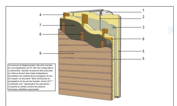
DEFINITION DES COMPOSANTS DE LA PAROI CONFORMES AU CGM DU NF DTU 31.2 ET NOTAMMENT AUX VALEURS CI-DESSOUS
